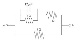
The circuit shown above has a constant voltage between points *a* and *b*. The voltage has been flowing for a long time. What is the resistance of the circuit?
