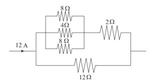
What is the voltage drop across the 12  $\Omega$  resistor in the portion of the circuit shown above?
