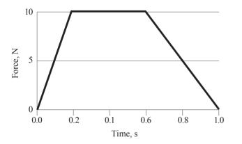
The graph above shows a force F acting on an object of mass m = 1 kg.
