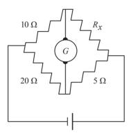
43. A Wheatstone bridge (diagram above) is a configuration of resistors and a sensitive current meter, called a *gal-vanometer*, that is used to determine the resistance of an unknown resistor. In the Wheatstone bridge shown here, find the value of  $R_x$  such that the current through galvanometer *G* is zero.
