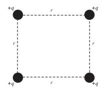
45. In the figure above, four charges are arranged. If the magnitudes of all the charges *q* are all the same and the distance *r* between them is as shown above, what is the magnitude of the net force on the bottom right charge in terms of *q*, *r*, and *k* (where  $k = \frac{1}{4\pi\epsilon_0}$ )?
