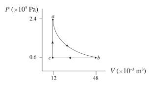
Path ab is an isotherm, and it can be shown that the work done by the gas as it changes isothermally from state a to state b is given by the equation
